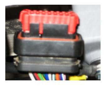
3. With red tab insert extended from housing (as shown above) pull the blue/white wire (pin 11) from the backside of the connector. Pin 11 is shown below (wire colors in pictures may not match).
