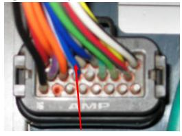
4. Now insert the wire into Pin 17 as shown below.
